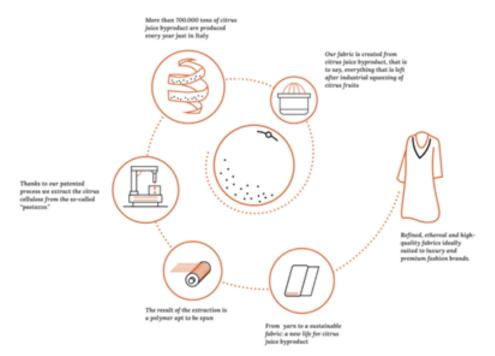
Process explained by Orange Fiber on how fabric is created from citrus juice byproduct (everything that is left after the industrial squeezing of the juice). Copyright Orange Fiber.
